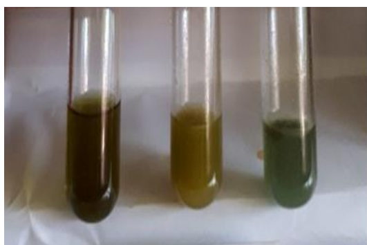
Figure 1. Flavonoid test (positive) a. samples before treatment; b. Samples after given NaOH 10% treatment; c. Samples after given HCl + Mg treatment)
